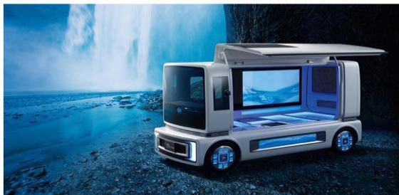
Figure 1. FC Show CASE (Anion Exchange Membrane Direct Hydrazine Fuel Cell Vehicle)
